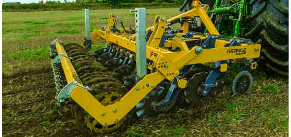
Grange's Strip-Till Preparator has been designed with input from farmers looking for the ideal tool to help establish their maize, sugar beet or brassica crops.
