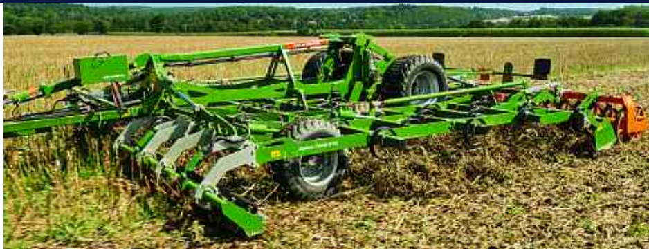
Amazone's Cobra was launched to meet the demands of the growing market for machines that work the top 5cm to help chit stubbles behind the combine.
