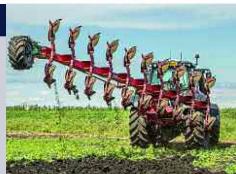
Bridging the distance between the plough and the cultivator, Kverneland's Ecomat On-land shallow has been designed for minimum disturbance seedbed preparation.
