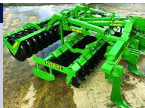
Cousins of Emneth's Patriot provides three working elements, including its front tines, followed by two rows of 50cm discs and the Razor Ring press at the rear.
