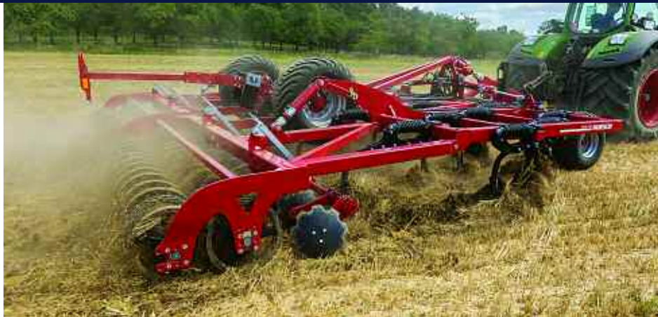
The Fortis 6 and 7 AS, have 6m and 7m working widths, respectively, and can operate with a working depth between 40cm and 30cm – aimed at deep loosening and primary tillage.
