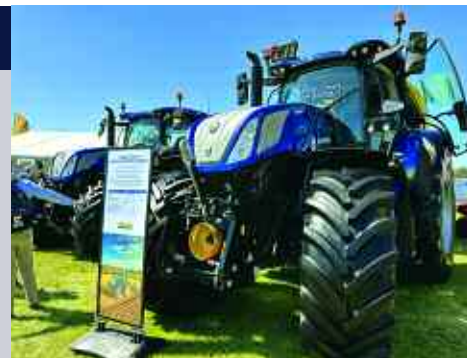
New Holland's new T7 340 tractor has a 6.7-litre NEF engine which delivers 340hp, plus it's been kitted out with a new sidewinder arm rest and 40cm monitor.
