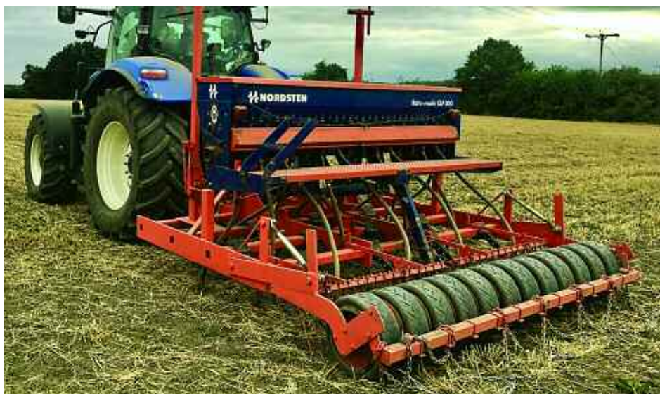
Coming in at a cost of around £4800, David Burton has made a bespoke direct drill using Metcalfe legs and tines.
