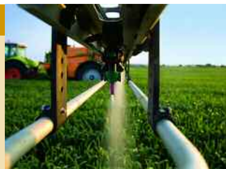
Nozzle type isn't just important but also size, because it has to deliver the water volume optimally.
