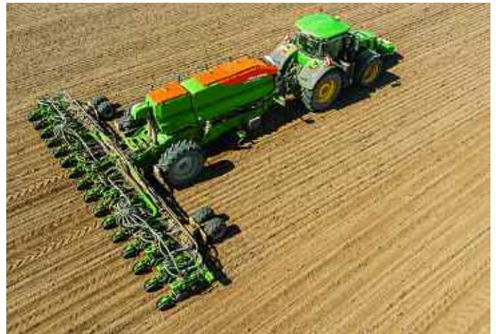
Amazone's Precea-TCC is offered with 12 or 16 rows at widths of 70cm, 75cm and 80cm.
