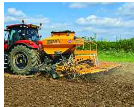
New this autumn is Mzuri's Pro-Til iGen - a one pass drill designed to produce an ideal seeding environment straight into stubble, cover crops and grassland.
