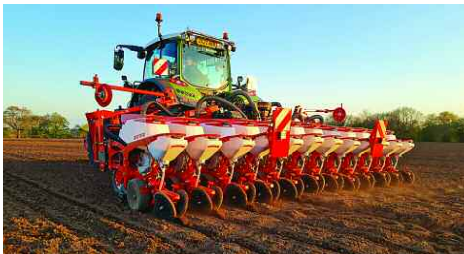
Maschio Gaspardo's Chrono 500 is a mounted machine which can be set up to run with variable row spacings and is equipped with either eight or 12 planting units.
