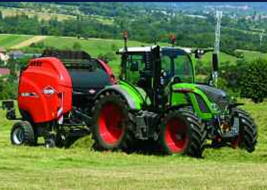
The VB 3285 is part of Kuhn's Strong range of balers and has a bale diameter ranging from 1.65m-1.85m.
