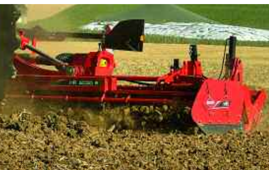
Kuhn's HR foldable power harrow is capable of working independently or in combination with a seedbar.
