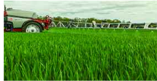
Booms on the Lexis 3800 include Kuhn Equilibra suspension technology which reacts to the way the boom moves, aiming to give three-dimensional stability.
