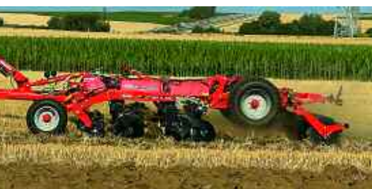
The Optimiser XL has 620mm discs and is designed to incorporate more trash, or for cover crop destruction, and can comfortably work down to depths of 15cm.
