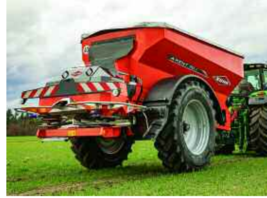
With a 9400-litre hopper capacity, the Axent 90.1 can spread up to 400kg/ha over 36m at more than 20km/h but can also work at widths of up to 50m.
