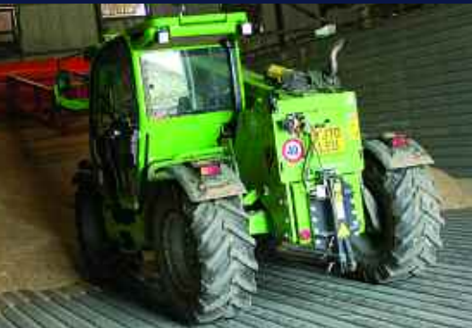
At 4.73m long, 2.31m wide and with a turning circle of just under 4m, Will rates the dimensions and manoeuvrability of the TF42.7.
