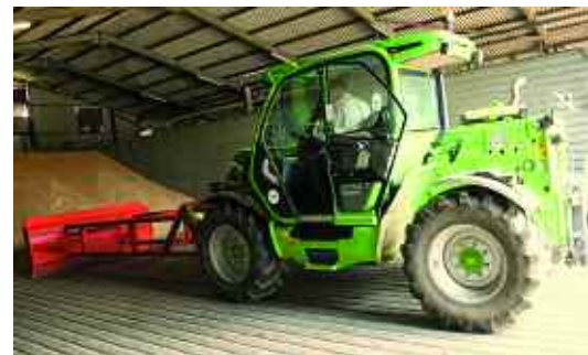
Will James relies on a pair of Merlo TF42.7 telehandlers to keep incoming trailer loads pushed up at harvest.
