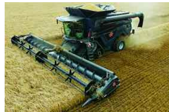
The farm's combine is a 12m-cut MF Ideal 9T, and with most land fairly close to the two main bases, trailers can come in at a high rate.
