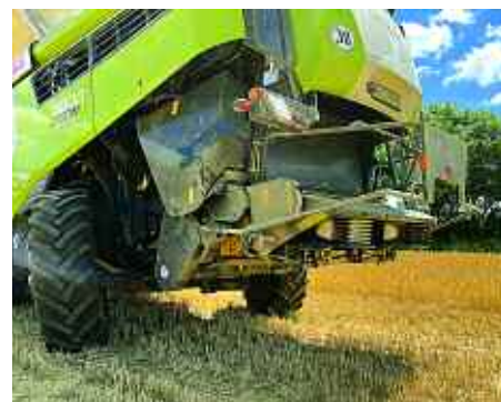
The seed control unit (SCU) is fitted below the straw chopper on the combine.
