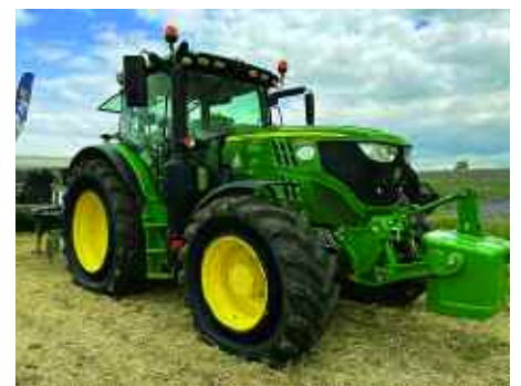
The CupWheel differs from conventional tyres because the V structure in the sidewall supports the lateral forces.
