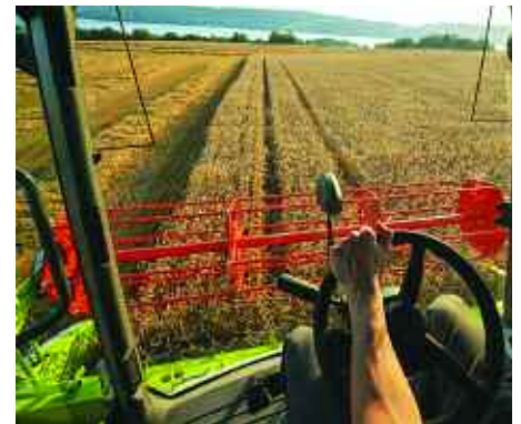
In the Claas Evion cab, there's a modern control armrest with the ergonomic Cmotion multifunction lever and the Cemis 700 touchscreen terminal.
