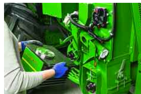
The sensor is fitted at the bottom of the grain tank elevator where grain is measured after it's been cleaned.
