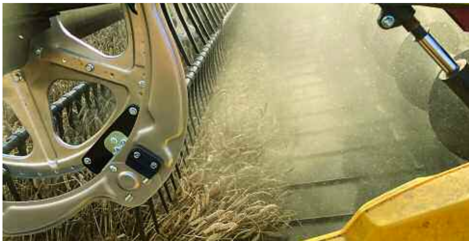
Longitudinal belts transfer cut crop heads-first across to the elevator feed belt.
