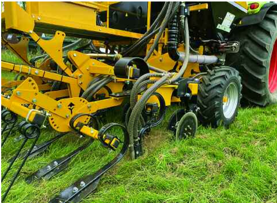
A 3m Claydon M3F with LD options drilling directly into a grass sward.
