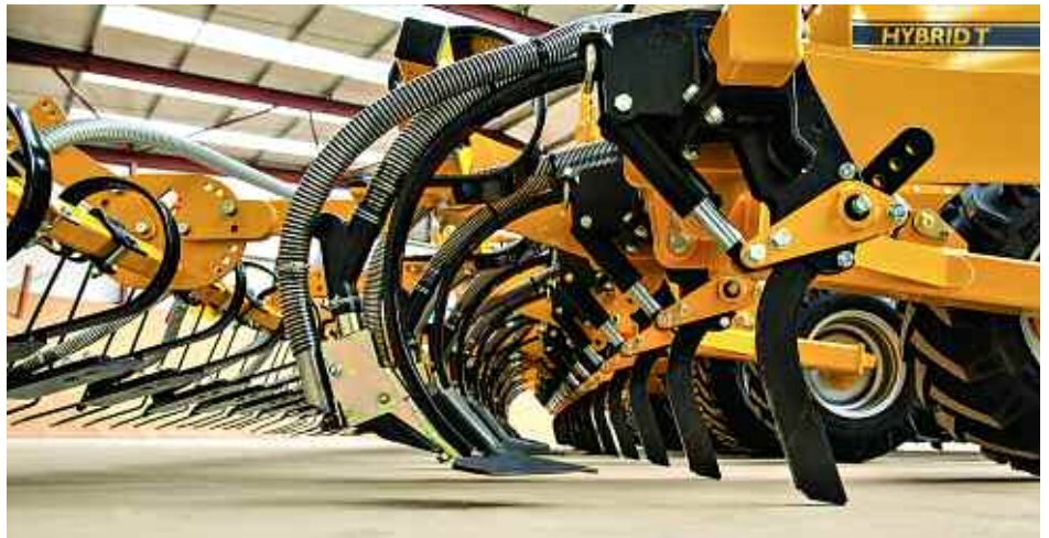
The Claydon Hybrid features a unique leading tine which is designed to move the optimum amount of soil, but only where required.
