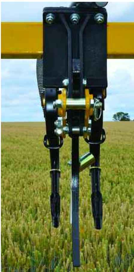
The two 44mm x 12mm hardened steel tines in the twin-tine unit are four times stronger than regular 30mm x 10mm tines.
