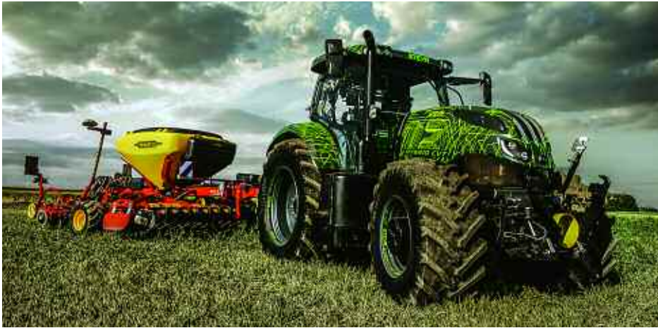
Steyr announced the launch of its hybrid CVT tractor in September. The tractor's E-CVT function means that this tractor is powered purely by hybrid-electric at up to 75kW and 1100rpm.
