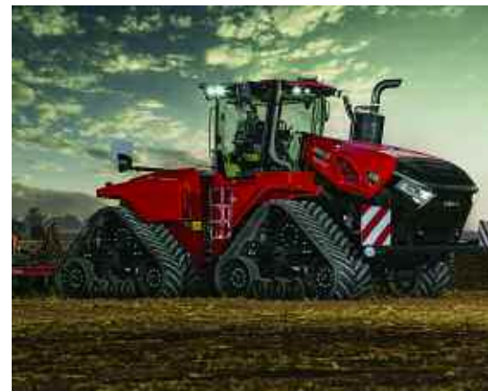
Case IH has now launched the new Quadtrac 715, boasting up to 778hp from a 16-litre FPT Cursor engine with two-stage turbo.
