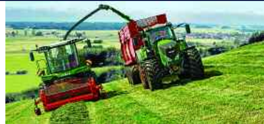
The Fendt Katana 650 achieves a rated power of 650hp with N MTU six-cylinder in-line engine.
