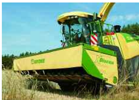
Krone's Big X is available from 480hp to 630hp with a 63cm width chopping drum, while the higher horsepower models, from 680hp to
