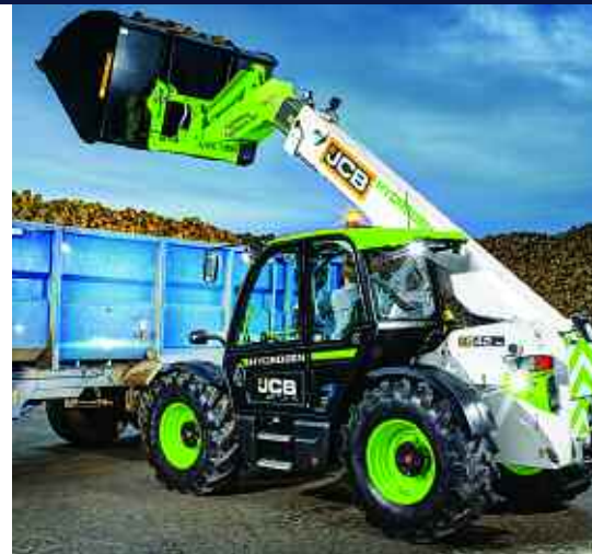
JCB has altered its internal combustion engine telehandlers and plant loaders to run off hydrogen without having to develop an entirely new fuel cell.
