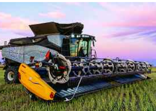
New Holland's CR11 combine has been designed for high-capacity harvesting, boasting a 775hp C16 engine and 5x61cm rotors.
