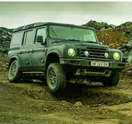
The Grenadier's robust five-link front and rear suspension is tuned to deliver great levels of axle articulation and wheel travel. Its Eibach progressive rate coil springs offer flex, with 9° of front-axle articulation and 12° at the rear – enabling more than 585mm of travel to maintain grip and make light work of driving over extreme uneven ground.
