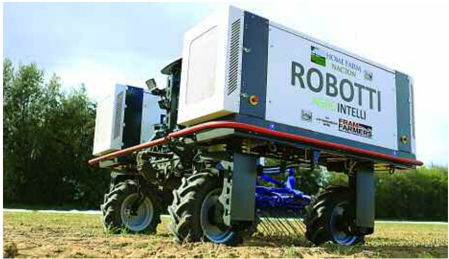
The Robotti has been fitted with a number of safety features, including a red stop bar and a LIDAR system so it'll come to a stop if an object gets too close.
