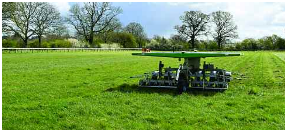
The FarmDroids rely on a base station on the farm for data transfer and everything from seed spacings to how close the weeding knives get to the plant can be controlled.
