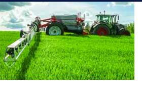
Pulse width modulation allows users to adjust the droplet size from the cab and provides turn compensation so that there's an equal dose across the width of the boom.
