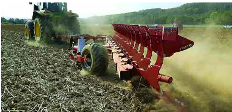
Ovlac's Eco Plus short bodies work at 8cm/3.5in to 25cm/10in, producing sufficient inversion to completely turn the soil and bury trash and weed seeds.
