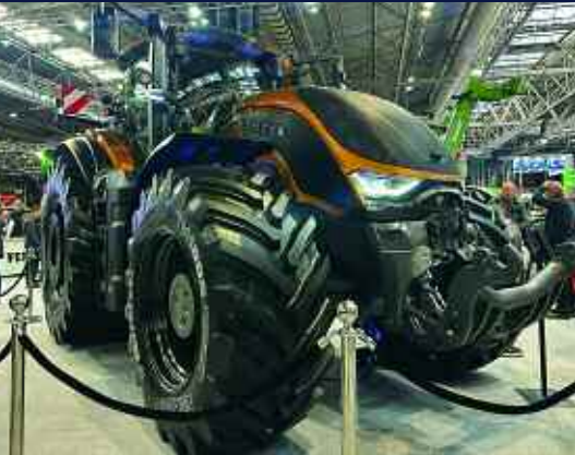
Valtra's new flagship sixth generation S Series - dubbed 'The Boss' by the firm - is its most powerful tractor, featuring an 8.1-litre AGCO Power engine.
