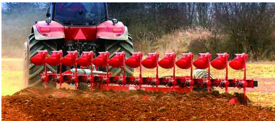
Reducing ploughing depth directly correlates to reduced power requirement and fuel use, so that halving the first cuts the latter two by 50% apiece, points out Ovlac.
