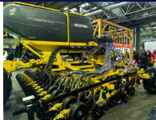
Another first for LAMMA 2024 is the Bednar DIRECTO NO 6000 which has been specifically designed for direct seeding of various crops.
