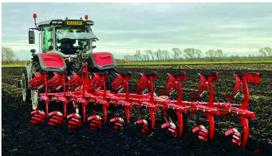
The shallow working depth of the plough promotes the development of cavities where air and water properly decompose the straw that's been mixed with the soil particles, claims Ovlac.
