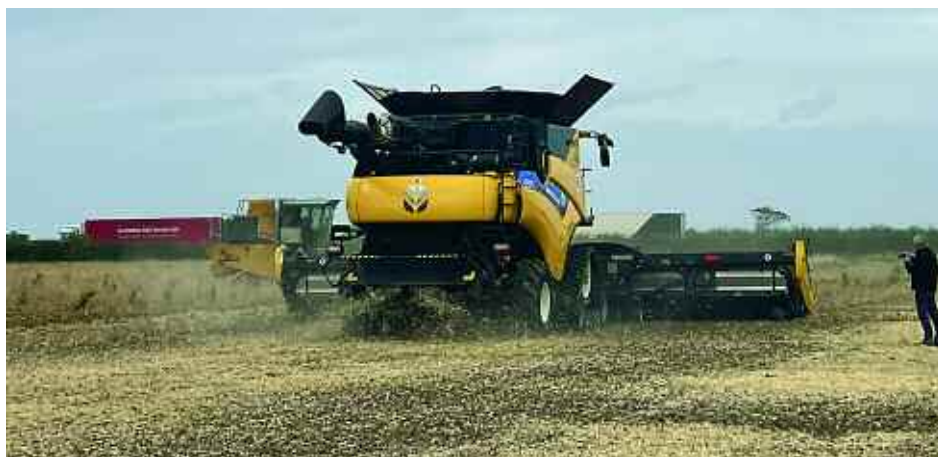
Capulet has proved difficult to combine until the introduction of the MacDon FlexDraper header which is able to combine the crop with minimal losses.
