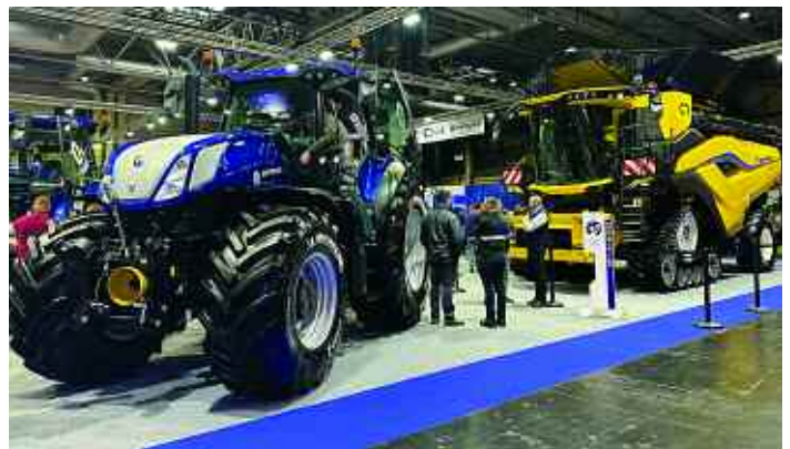
New Holland's new flagship combine the CR11, features a 775hp C16 engine, two 61cm rotors, a 20,000-litre grain tank and a 210litre/sec unload rate.
