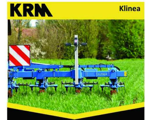
The Klinea is the latest innovation in cereals hoeing. It features central tine angle adjustment (without tools) to improve penetration in hard conditions and utilises the new Kipline camera system for automatic guidance. The shares are followed by harrow tines to remove soil from weed roots and prevent re-growth. Optional section control lifts each element independently at the headland for the ultimate in accuracy and efficiency.
