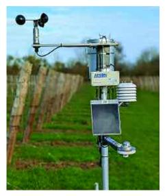
Several hundred weather stations provided by Agrovista are in use across the UK, measuring a range of parameters including rainfall, air temperature, soil temperature and soil moisture.
