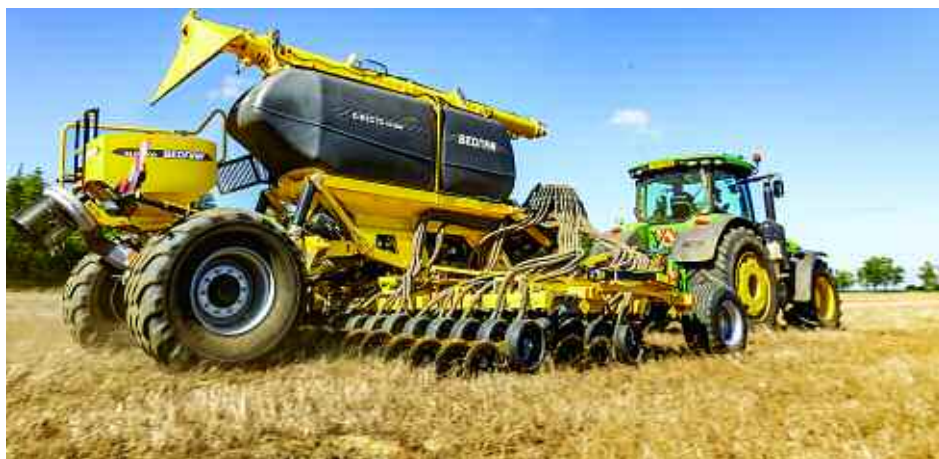
Bednar's Directo No is equipped with a double-chamber pressurised hopper with a 5000-litre total capacity and can be used for a single crop or dual application with fertiliser.
