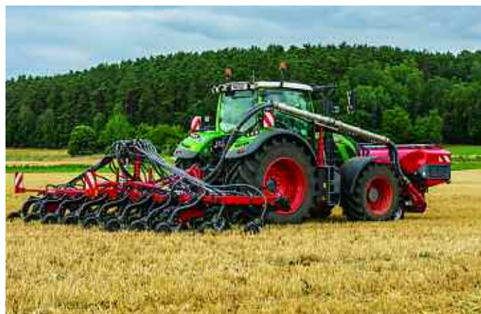
Two new models join Horsch's popular Sprinter tine seed drill range – the Sprinter 6.25 SL and 12.25 SC. The models are aimed at reducing tillage to a minimum but can work well in high amounts of straw residue.
