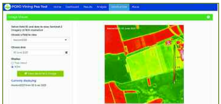
The machine learning is combined with satellite data which provides the platform with multispectral canopy reflectance measurements, derived from the Sentinel-2 system.
