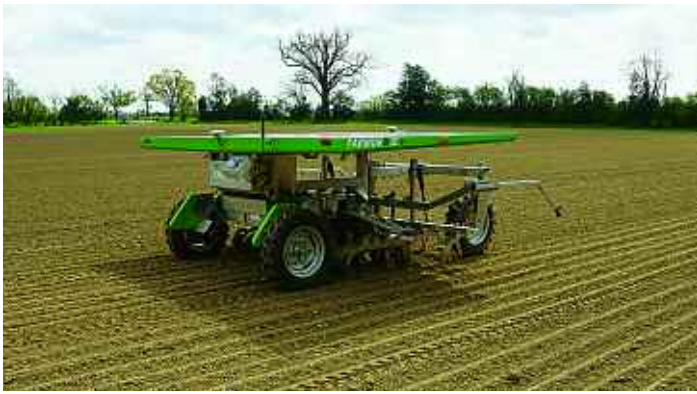
A four-wheeled version of the FarmDroid has been launched to allow it to straddle rows of crop, enabling it to plant seed into flat beds and return subsequently to weed between the seedlings without running any crop down.
