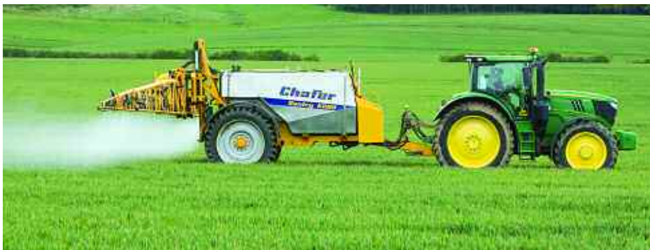
Applying a T1 spray will help to stop the spread of disease above leaf three, protecting 75% of the yield which is produced by the top three leaves and the ear.
