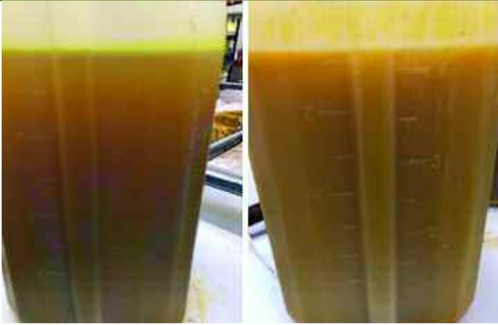
*In some cases, it may be possible to recover problematic tank mixes with Kantor. The left image shows an incompatible 7-way mix experiencing phase separation and sedimentation while the right image shows the solution fully mixed after the addition of Kantor.*
