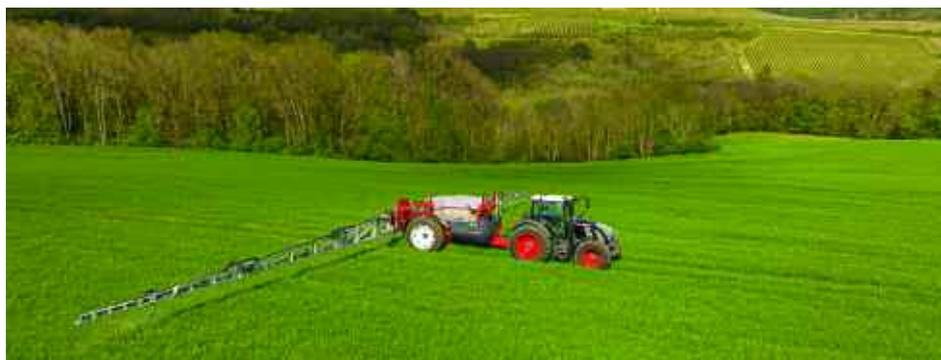
*To manage droplet size more effectively on Kuhn's Metris 2 trailed sprayers, Autospray pulse width modulation (PWM) offers continuous high-pressure circulation to enable precise operation with each nozzle.*
