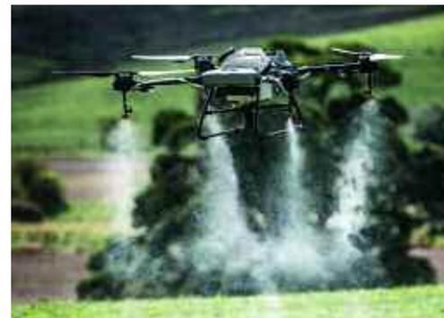
*This year Drone Ag's planning to conduct a few different trials in the UK including glyphosate spraying, which means drones may soon be utilised to their full capacity.*
