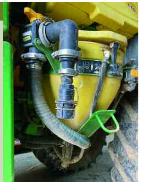
*Specifically designed parts were used to connect the CTS to the sprayer.*
