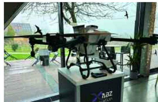
can also be used directly after rain because ground travel isn't prohibited," he adds. "Legislation means that spraying can't be done in wind speeds of more than 5m per second, but our drones are theoretically able to spray safely in wind speeds of 7-8m per second if the speed and altitude of the drone is reduced. However, in terms of being able to fly safely, the drones can handle winds of up to 20m per second."
