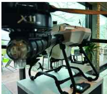
Propellers on the drone provide strong downforce, and when optimised, can create uniform spray patterns.
