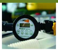
CTSs improve product measuring precision, with the FasTran 850 bringing flow accuracy to within +/- 0.5% while dispensing 25 litres/min.
