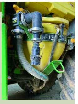
Specifically designed parts were used to connect the CTS to the sprayer.
