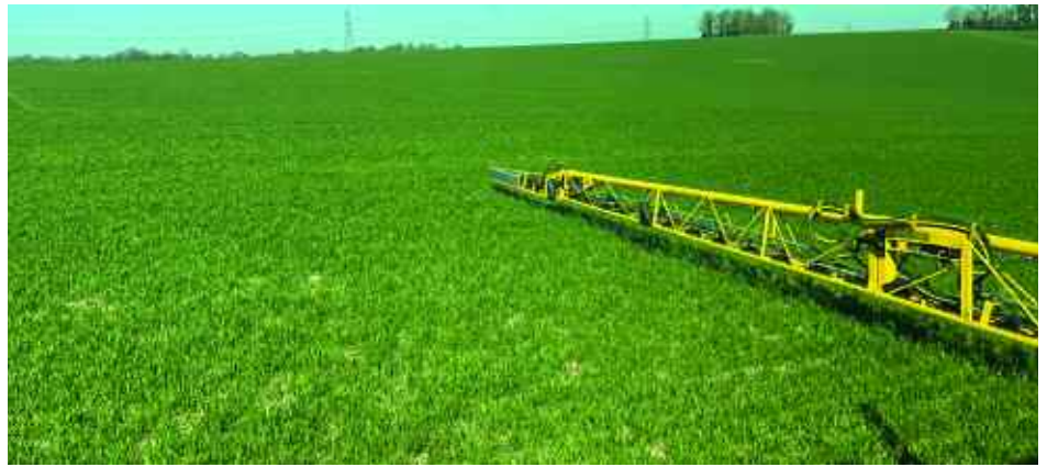
The Interceptor is fitted with a Gen 2 Raven Hawkeye system, which operates individual nozzle shut off and individual nozzle rate control.
