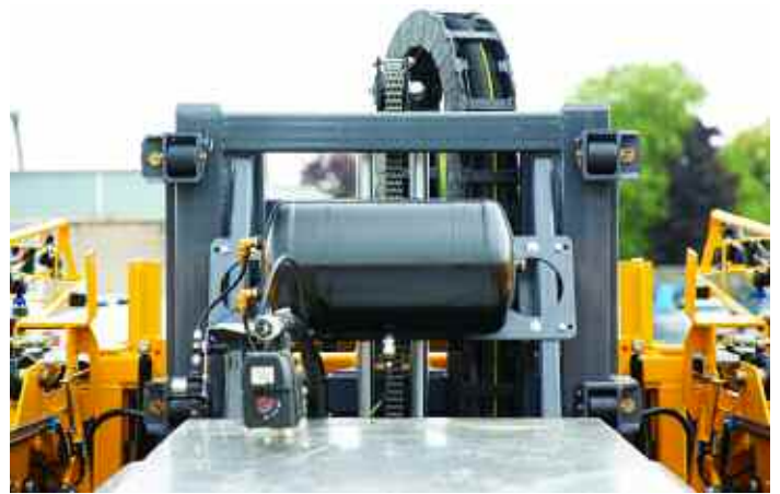
Air Purge – part of the ePlumbing system – uses compressed air to blow all but about 3 litres of residues out of the boom.
