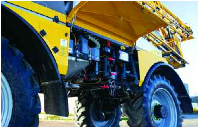
The ePlumbing system detects if valves are open or closed and also to the nearest degree.
