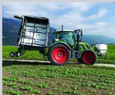
The Ara consists of three 2m wide enclosed compartments, totalling 6m in width which can be folded to 2.8m for road transport.
