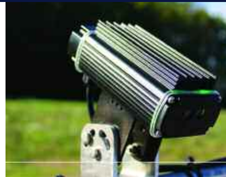
Kuhn has continued to test and develop its spot spraying system – I-Spray with both 'green on brown' and 'green on green' weed detection possible, offering up to 95% savings in chemical products.
