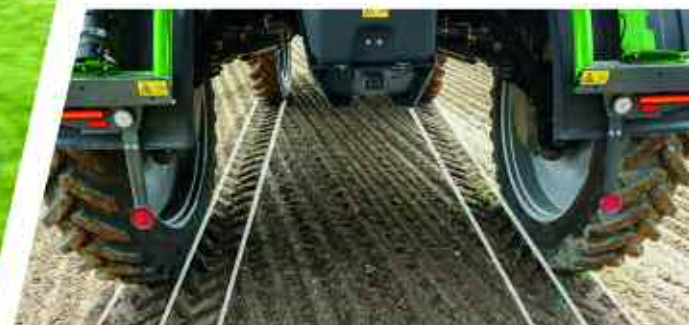
Offset track width driving helps minimise soil compaction.
