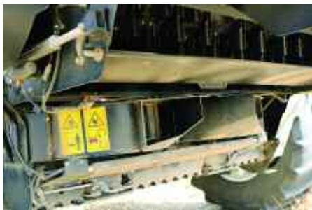
The Redekop SCU is claimed to destroy 98% of the weed seed that passes through it.
