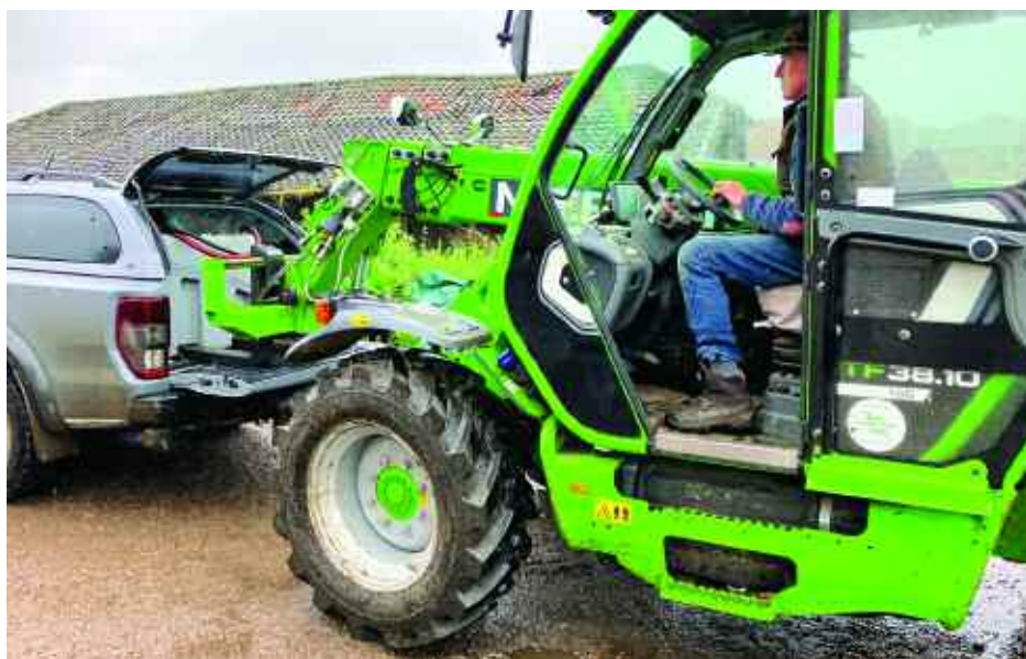
Merlo's infinitely-variable hydrostatic transmission provides the smooth response necessary for delicate loading tasks, says Geoff Mayhew.
