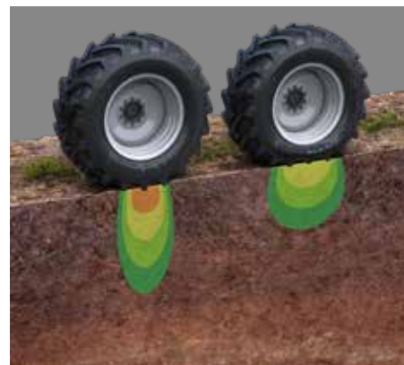
VF tyres provide the ability to carry 40% more load at the same pressure as a standard tyre, or for the machine to run at 40% less pressure than a standard tyre when carrying the same load.
