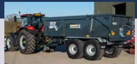
The MP18 body is constructed from Hardox steel to reduce weight and increase strength, while enhancing wear resistance above the high-grade steel used in the Richard Western's other trailers.
