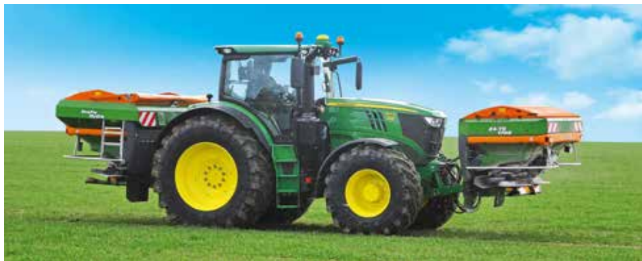
Spreading technology has advanced significantly in the past 40 years, with machines now able to adjust for wind speed and direction, modify spread at headlands and utilise spread pattern radar.
