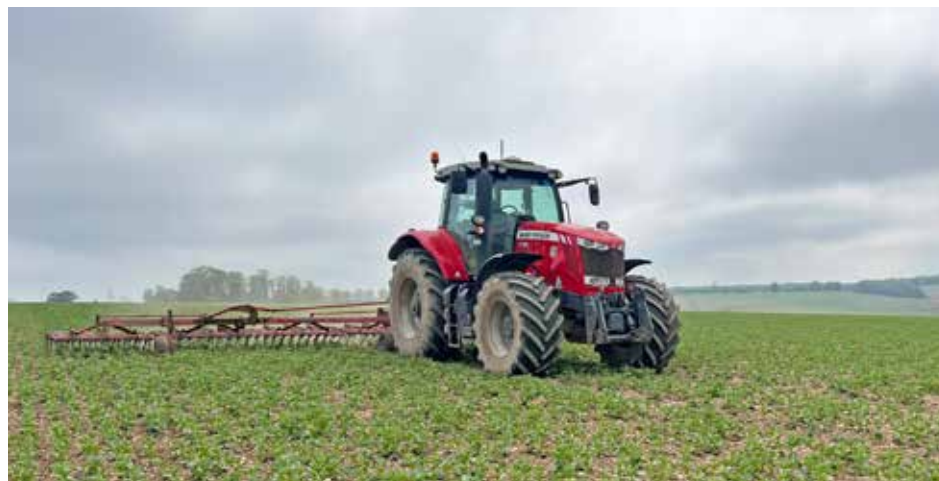
To keep weeds at bay, a scratcher harrow is used when crops are about an inch from emergence, followed by two or three passes with the weed harrow before the crop gets too tall.
