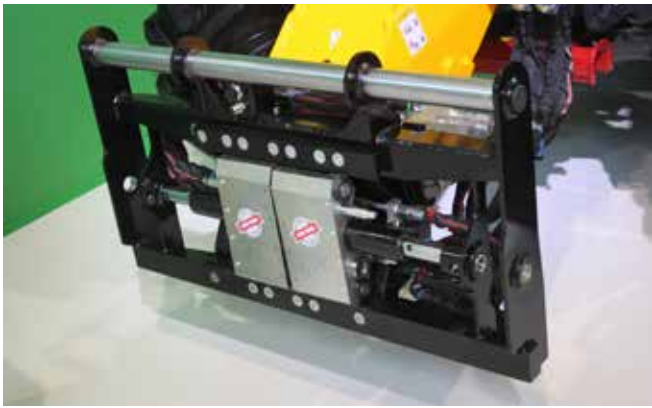
The Fast-Attach system from Dieci is said to be the only system available which connects all mechanical, hydraulic and electrical couplings.
