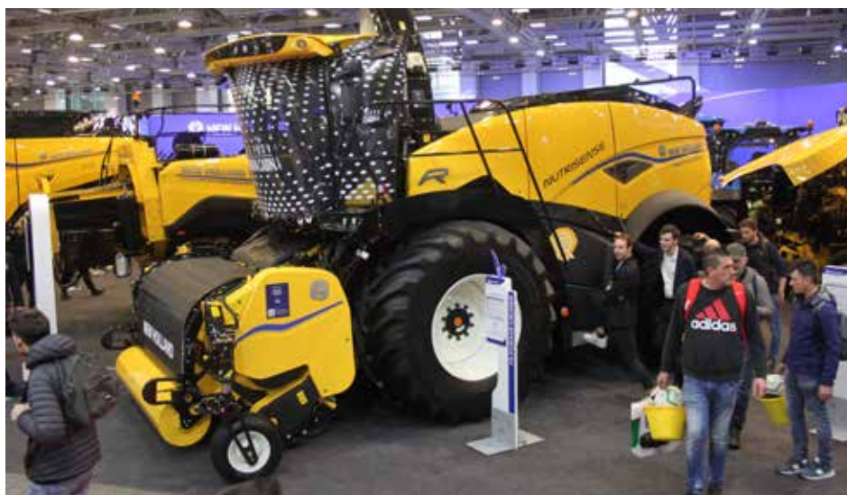
The CropSpeed system on New Holland's latest FR Forage Cruiser self-propelled forage harvesters uses a spout-mounted radar to monitor crop flow and reduce blockage risk.
