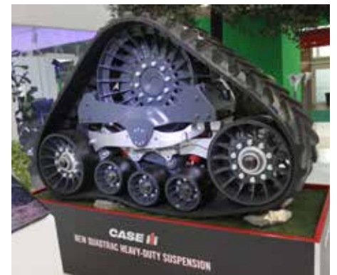
The new Case IH Quadtrac track suspension system is said to enhance operator comfort, track footprint, workrates and implement performance.
