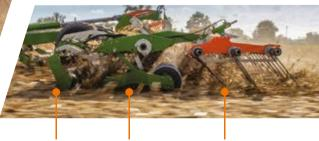
First row of optional leading tools: **Knife roller**  Second and third row main tools: Combination of knife roller and/or Minimum TillDisc
