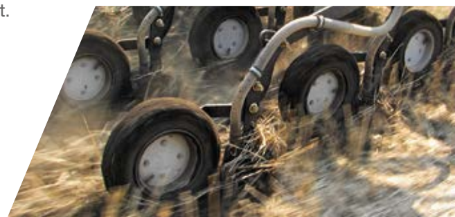
The ConTeC pro opener ensures the perfect seed placement.
