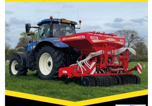
KRM GS300 drills feature rubber mounted, 400mm notched disc coulters are ideal for working directly into existing grassland. The prism roller provides excellent closing of the seed slot ensuring seed to soil contact for rapid germination and growth. The electrically driven central metering unit can handle all seed types and sizes making it ideal for introducing companion crops and establishing herbal lays.
