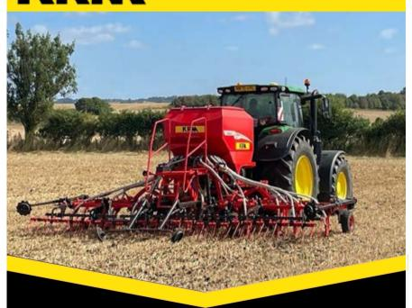
KRM SM-P tine drills qualify for the latest round of FETF Grant Funding. The heavy duty SM coulters with their narrow carbide tip are ideally suited to direct drilling or sowing into min-till seedbeds. The ISObus controlled electric metering system is fed from the pressurised hopper for accurate sowing rates from 4-400kg/ha. Available in working widths up to 8m and with wide spaced options available to compliment mechanical weeding solutions also available at KRM.
